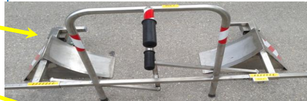
SBCoupling before emergency disconnect
